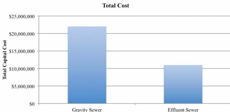
Chart 1. Capital cost of gravity sewer versus effluent sewer.
