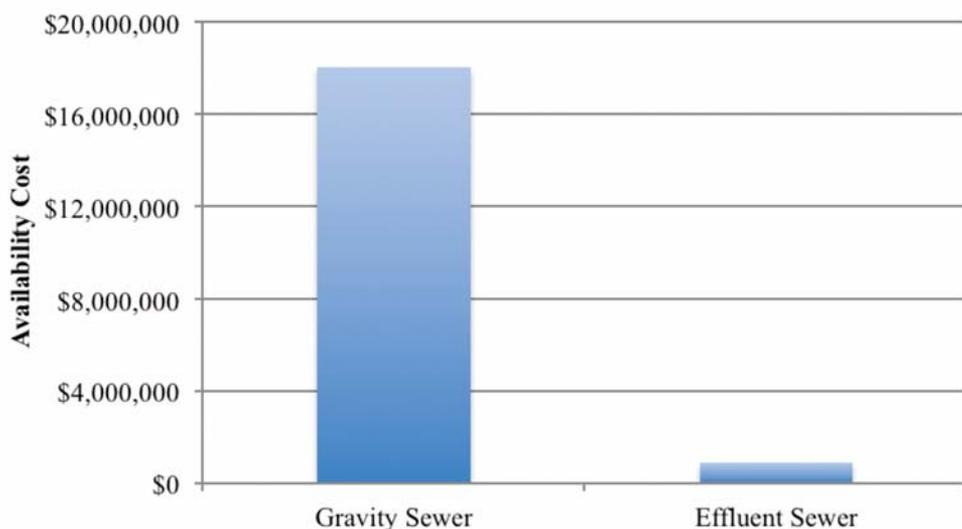
Chart 2. Availability cost of gravity sewer versus effluent sewer.
